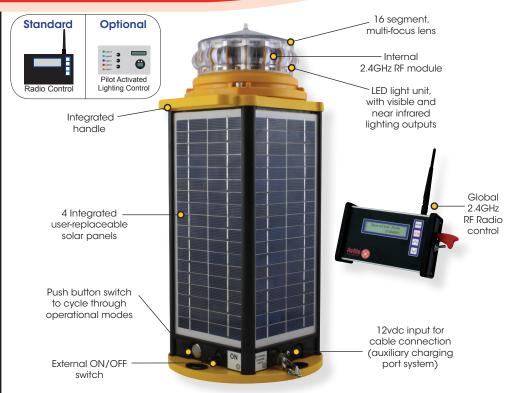
The AV-425-RF is a robust, completely self-contained LED light designed for a range of emergency aviation applications including runway, threshold, approach, helipad and tactical airfield lighting. Fitted with RF radio control, this fully functioning light can be controlled from the tower with no costly cabling or trenching required.
